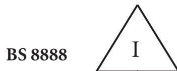
**Figure 4:** Method of indicating that the independency system of tolerancing has been used
