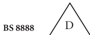
**Figure 5:** Method of indicating that the dependency system of tolerancing has been used
