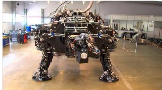
A 2.0 liter diesel powered autonomous robot.
